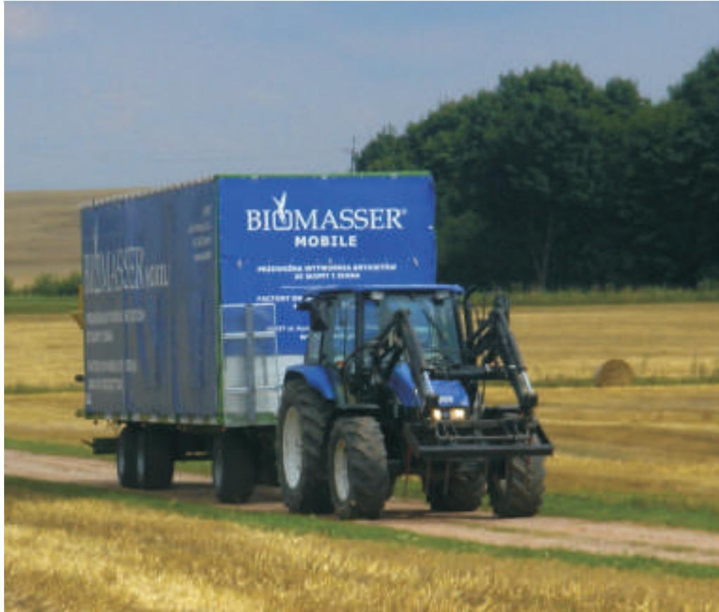
BIOMASSER® MOBILE is a transportable production line which may be conveyed to the location of raw materials store. This allows customers to eliminate the high transportation costs normally associated with moving straw to a place of briquette production. Moreover, it is suitable for executing a briquetting service for a customer.
